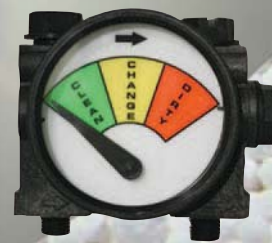
Differential Pressure Gauge
