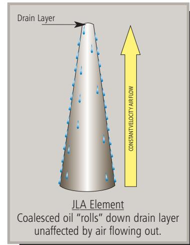
Annular velocity remains low and constant in direction of flow.
